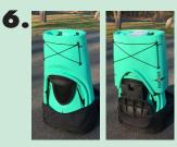
Place section 4 on 2. Before placing section 3 on 4, make sure foot pedals are all the way down toward bulkhead and locked. Flip the cockpit pad over the clamps so they don't scratch section 4.
